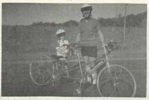
of my 50-pound stoker and me. I used Specialized Touring K-4 tires because they are supposed to be puncture resistant, and though the wheels are quick-release, they aren't especially easy to remove and replace.
