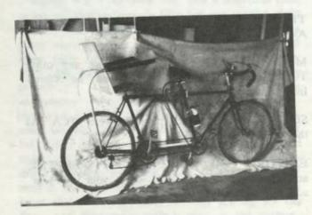
Being both handy and mildly obsessive, I built such a rig for my daughter and our ancient Jack Taylor. Lacking welding or brazing equipment, I made a clamp out of cherry to hold a typical handlebar stem upright in the middle of the stokers
