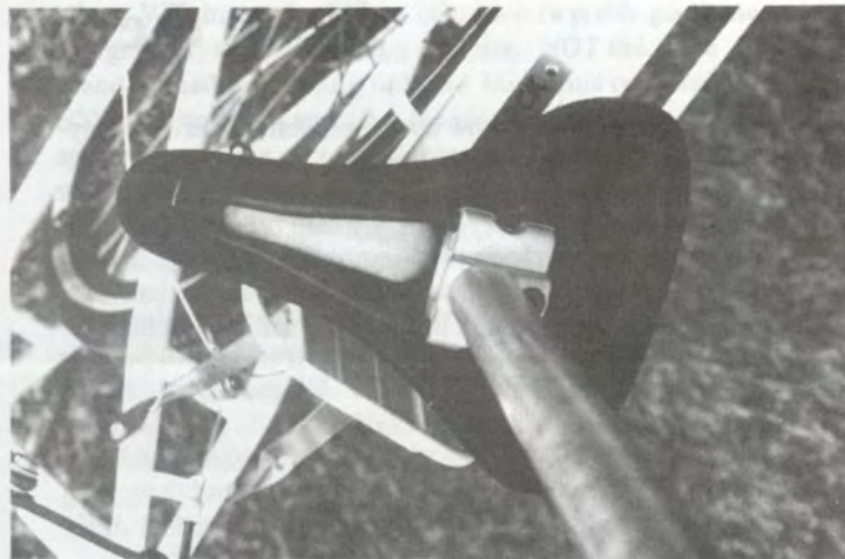
The Underside of the Terry Saddle, showing the cutout.
