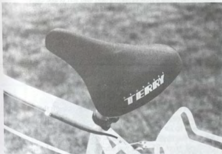
The Terry Saddle. Note the depression where the foam changes density.
