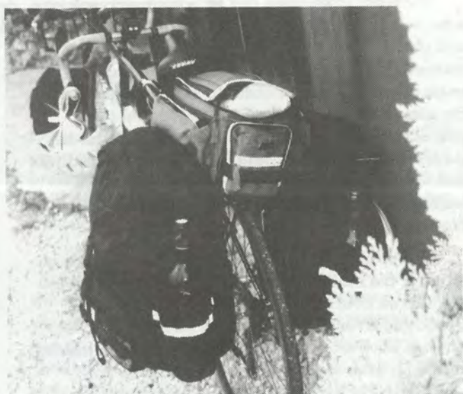
The well packed tandem. Note the importance of the vertical rear pockets on the panniers.
